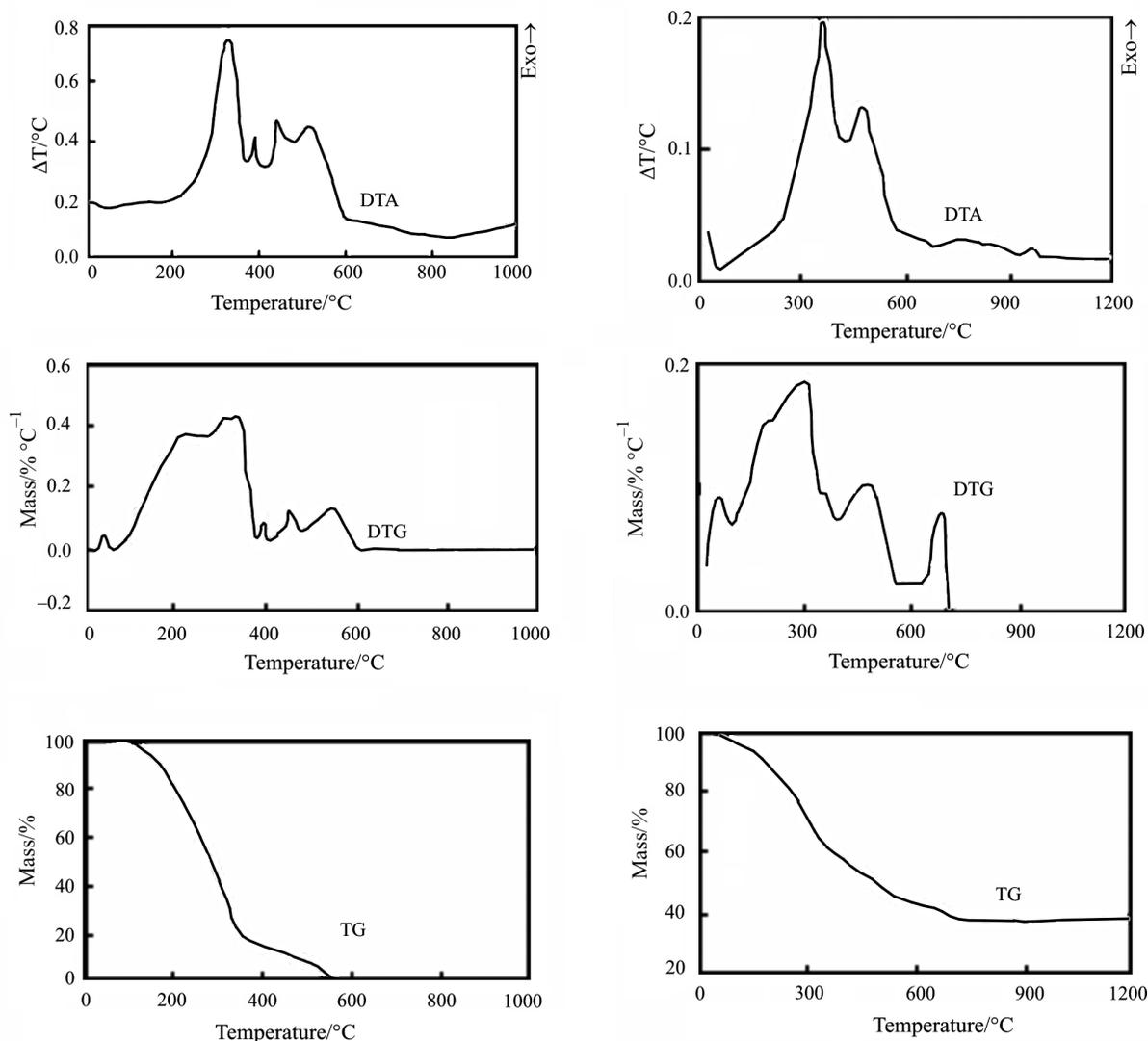
Fig. 1 Thermal curves of SOM and sludge
