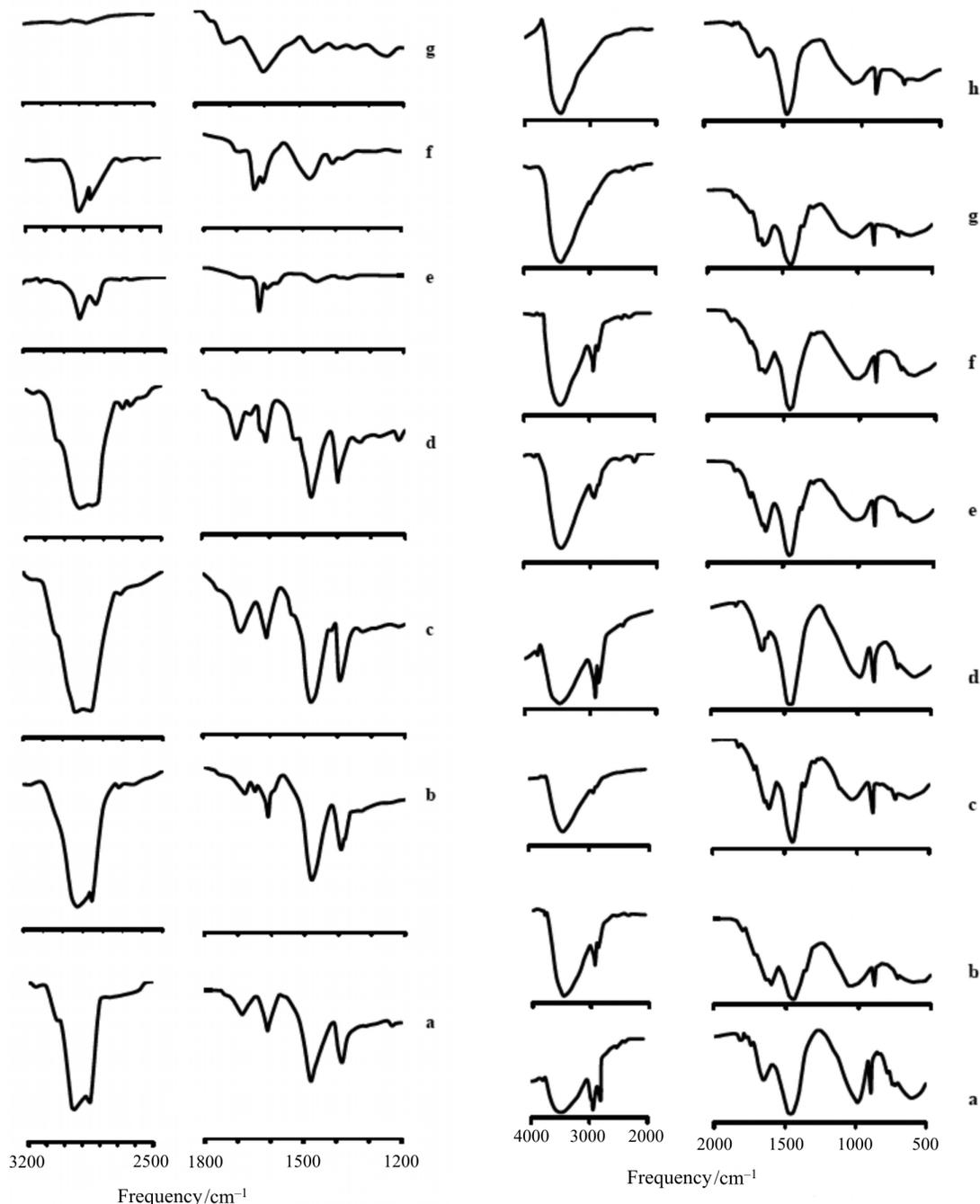
**Fig. 2** IR spectra of SOM and FTIR spectra of sludge, heat treated at different temperatures and times: a – original; b – 250°C for 0 min; c – 250°C for 60 min; d – 350°C for 0 min; e – 350°C for 60 min; f – 450°C for 0 min; g – 450°C for 60 min; h – 550°C for 0 min (sludge only)
