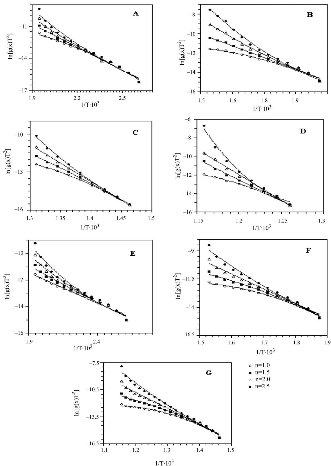
**Fig. 3**  $1/T \cdot 10^3$  ( $K^{-1}$ ) vs.  $\ln[g(x)/T^2]$  plots for SOM (A, B, C, D) and sludge (E, F, G) at different temperature regions: (A, E) 100–250°C, (B, F) 250–400°C, (C) 400–500°C, (D) 500–600°C, (G) 400–600°C
